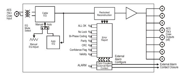
Figure 1-2. AES-6880 Functional Block Diagram
